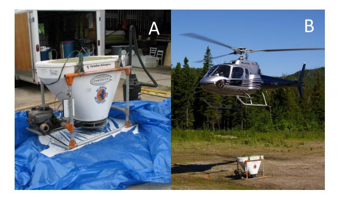
Figure 2. Equipment used for the dry application of the pheromone flakes. A) the speader; B) The helicopter under which was attached the spreader.
